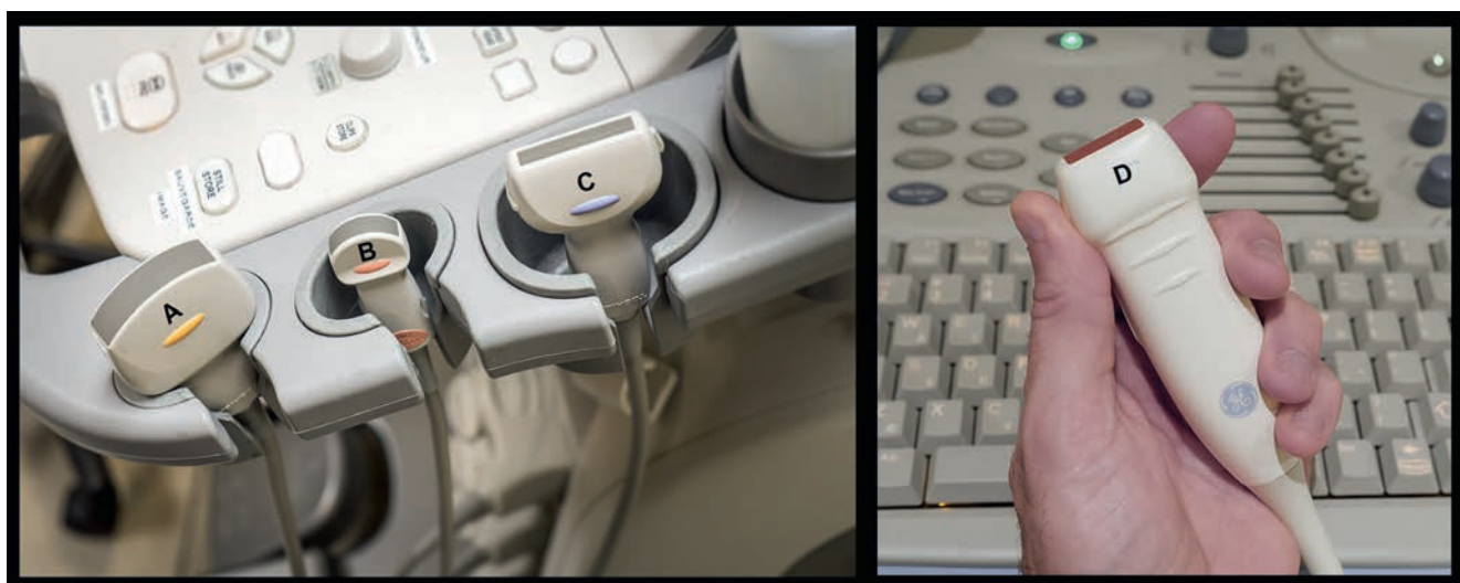
Figure 1.4. Practical ultrasound transducers. Most ultrasound units are equipped with convex (A, B) and linear (C) electronic transducers with variable frequencies. A macroconvex probe offering lower frequencies (3–8 MHz) is best suited for the abdomen of large dogs, whereas a microconvex probe (B) of higher frequency and smaller footprint is preferred for the abdomen of small patients and when only a small acoustic window is available (e.g., intercostal approach of a lung lesion). A high-frequency (10–18 MHz) linear probe is most useful for assessing superficial structures on a relatively wide and flat surface (e.g., assessing bowels in a cat, biceps tendon in a dog). A phased array transducer (D) offers a small flat footprint and is ideal for echocardiography.
